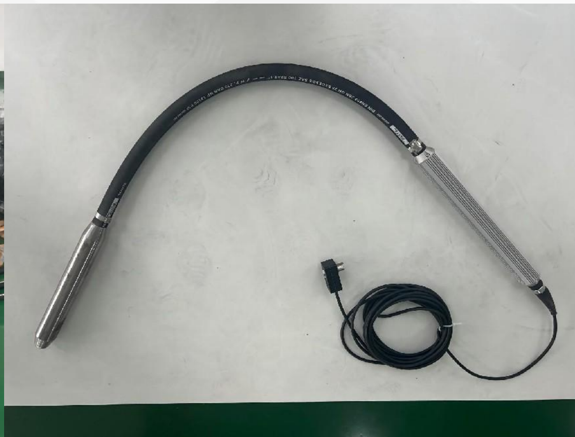
Completed Vibrator rod unit
